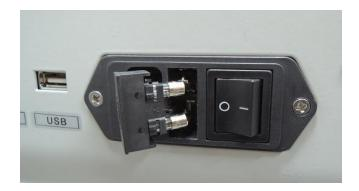
4) Take out the disconnected fuse from the fuse slot, and replace it with a new fuse with the specification of 250V, F6.3AL, 5×20mm.
