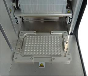
15) Insert elution cartridge into elution heating block.
