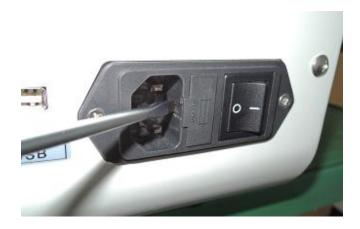
3) Pull out the fuse slot and check the condition of fuses.
