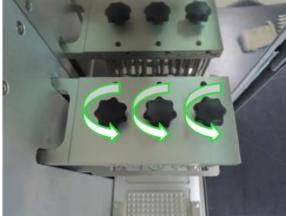
3) Remove the bracket at the top of the magnetic rods plate by turning it to the left.
