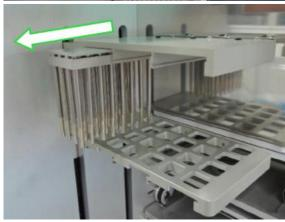
4) Pulling the magnetic rods toward the front of the instrument will remove the magnetic rods.
