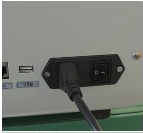
1) Connect the power cord to the back of the instrument and approve the power source.
