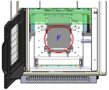
8. Open the door and remove the **Sponge block (F)** from the Base Plate after initialization.
