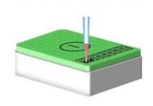
7. Load samples into the **'Sample Loading Well'** of Buffer Cartridge ①.
