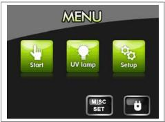
1. Press the 'Setup' button to access the SETUP menu.
