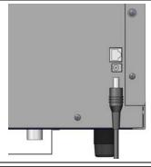
5. Connect the power cable to the rear of the instrument.
