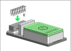
3. Make sure you have purchased the correct kit for the sample type and target nucleic acid type you desire. Insert the desired number of **Elution tubes (E)** into the Elution Tube Rack.
