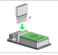
4. Insert the **Disposable Tips (F)** into the Disposable tip rack in the same quantity and relative position as the Elution tubes.
