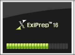
7. Press the power button on the LCD screen to initialize the instrument. A progress bar on the lower portion of the LCD touch-screen will indicate initialization progress.
