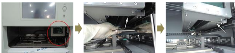
Fig. 52 Decontamination step-1 ; Separation and installation of the Contamination Shield
