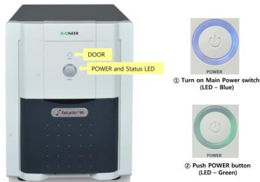
Fig. 42 Operation button (door button, power button and status LED) of Exicycler™ 96
