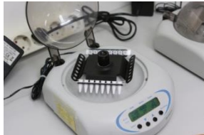
Fig. 41 Mix the PCR Premix Strip using ExiSpin™
