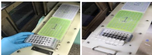
Fig. 24 Inserting the Disposable Tips into the Disposable Tip Rack
