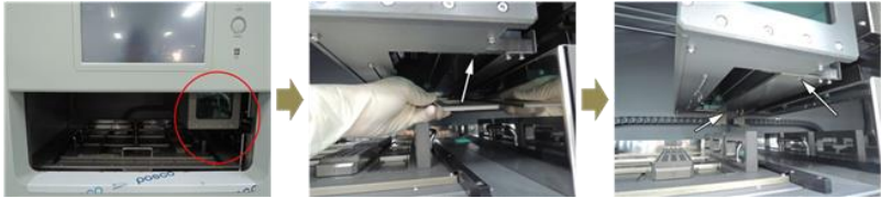
Fig. 51 Decontamination step-1 ; Separation and installation of the Contamination Shield
