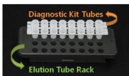
Fig. 57 Checking the position of diagnostic kit tubes in elution tube rack
