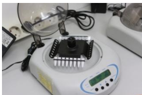
Fig. 41 Mix the PCR Premix Strip using ExiSpin ™
