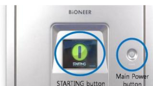
Fig. 5 Starting button and main power button of ExiPrep™ 16 Dx
