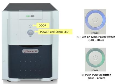
Fig. 42 Operation button (door button, power button and status LED) of Exicycler ™ 96
