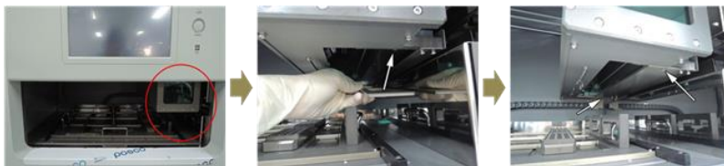
Fig. 50 Decontamination step-1 ; Separation and installation of the Contamination Shield
