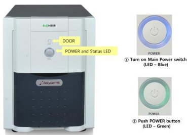
Fig. 41 Operation button (door button, power button and status LED) of Exicycler ™ 96
