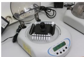
Fig. 40 Mix the PCR Premix Strip using ExiSpin™
