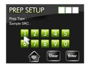
12. The PREP SETUP screen appears as shown in the left, press protocol number according to the protocol number list (pp. 12-14). Confirm following information displayed on the screen, and then press the 'Enter' button.
