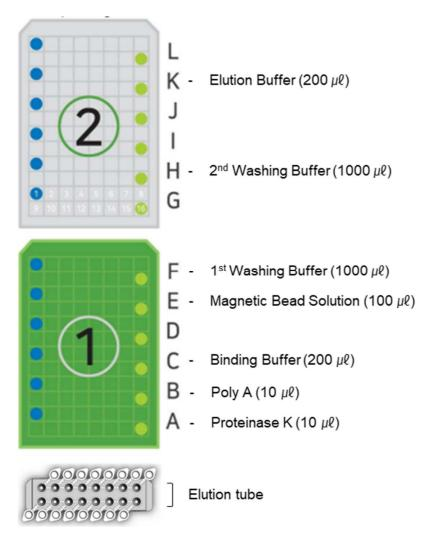
Figure 1. Position of reagents, tubes, and starting material in Cartridges/Elution Tube Rack of *ExiPrep*<sup>™</sup> Plus Viral DNA/RNA Kit (K-4271), *ExiPrep*<sup>™</sup> Plus Viral DNA Kit (K-4272), *ExiPrep*<sup>™</sup> Plus Viral RNA Kit (K-4273).
