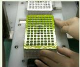
5. Place the Buffer Cartridge ① onto the proper position of the baseplate.
