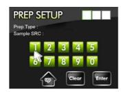
12. The PREP SETUP screen appears as shown in the left, and a screen to select the protocol number for each kit appears. Press <u>'204' or '205'</u> according to sample type. Confirm following information displayed on the screen, and then press the 'Enter' button.
