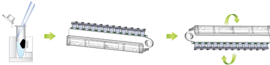
Figure 5. Washing the beads to remove residual ethanol.
