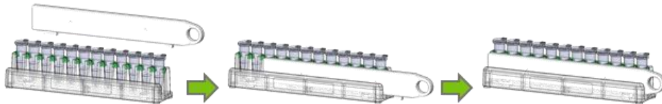
Figure 2. Attachment of the Magnet plate. Combine the magnet plate to the stand.
