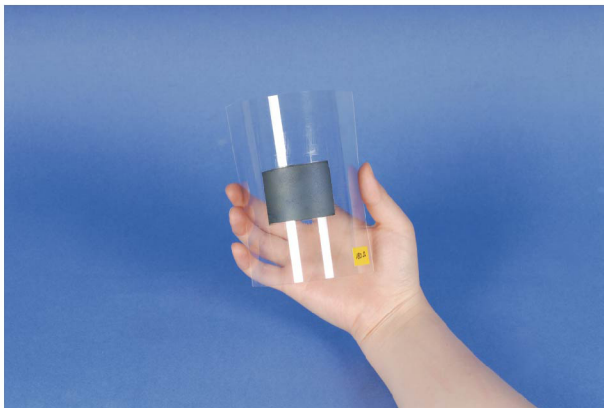
Figure 7. PET film printed with CNT-Ag paste and increased temperature to 150 °C The Temperature lasts 2 hours for melting of silver nano particles on Carbon Nanotube. Electrical conductivity of CNT-Ag printed on PET film is 2.5 \times 10^{-2} S/cm.
