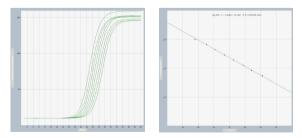
**Figure 5.** Fluorescence data from a series of 1.33-fold dilutions of TMV gene (10<sup>6</sup> copies) amplified using reporter dyes to check one target: FAM/TMV. The PCR efficiency generated by the standard curve is 101%.
