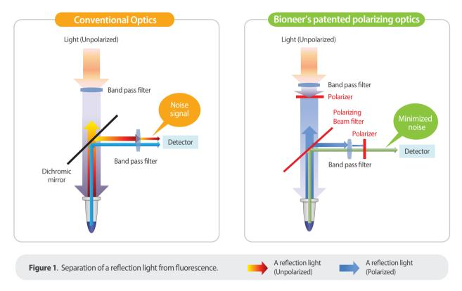
\* Problem of a reflection light: In the conventional technology, excitation light is generally brighter than fluorescence generated from the sample. Therefore, light reflected from an optical component interferes with the fluorescence generated from the sample. Furthermore, it is hard to completely distinguish one from the other. This can cause imprecise and unreliable results.
