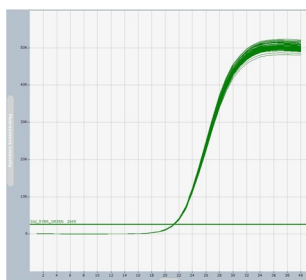
Figure 1. Excellent Uniformity Fluorescence data using 10^6 copies of IRF3 gene (FAM labeled) in each of 96 well positions. The average Ct of 96 well is 21.8 and the Ct variation range is 0.19.
