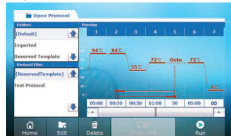
Figure 9. On the 'Open Protocol' menu, you can find previously saved protocols that are displayed instantly on the screen.
